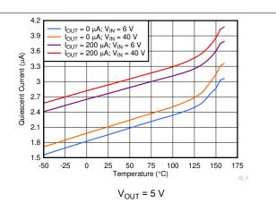
Figure 6-2. Quiescent Current vs Ambient Temperature
