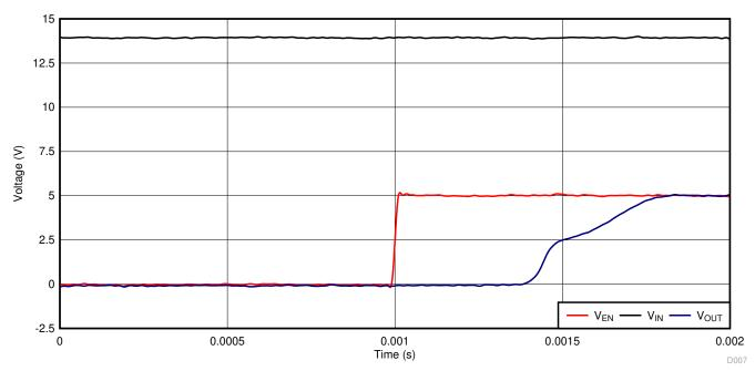
Figure 8-8. TPS7B81-Q1 Power-Up Waveform (5 V)
