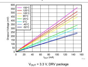
Figure 6-5. Dropout Voltage vs Output Current
