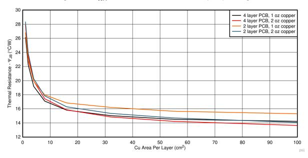
Figure 8-6.  $\psi_{JB}$  versus Cu Area for the TO-252 (KVU) Package
