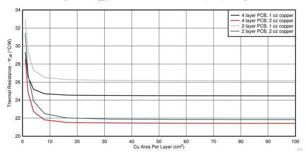
Figure 8-2.  $\psi_{JB}$  versus Cu Area for the WSON (DRV) Package
