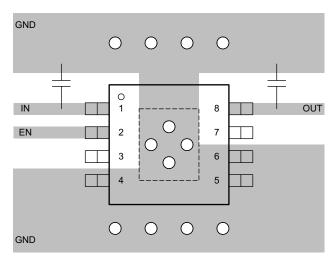
Figure 10-1. TPSB81-Q1 Example Layout Diagram
