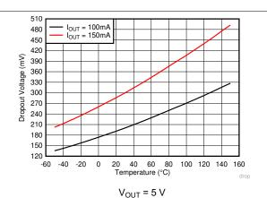
Figure 6-6. Dropout Voltage vs Ambient Temperature
