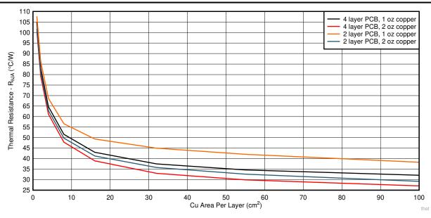
Figure 8-5.  $R_{\theta JA}$  versus Cu Area for the TO-252 (KVU) Package
