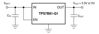
Figure 8-7. TPS7B81-Q1 Typical Application Schematic
