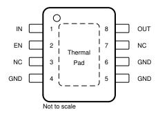
Figure 5-1. DGN Package, 8-Pin HVSSOP PowerPAD™, Top View
