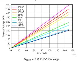
**Figure 6-4. Dropout Voltage vs Output Current**
