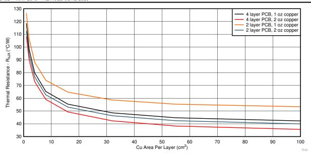
Figure 8-3.  $R_{\theta JA}$  versus Cu Area for the HVSSOP (DGN) Package
