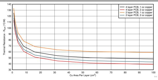
Figure 8-1.  $R_{\theta JA}$  versus Cu Area for the WSON (DRV) Package
