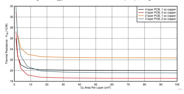
Figure 8-4.  $\psi_{JB}$  versus Cu Area for the HVSSOP (DGN) Package
