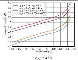
Figure 6-3. Quiescent Current vs Ambient Temperature
